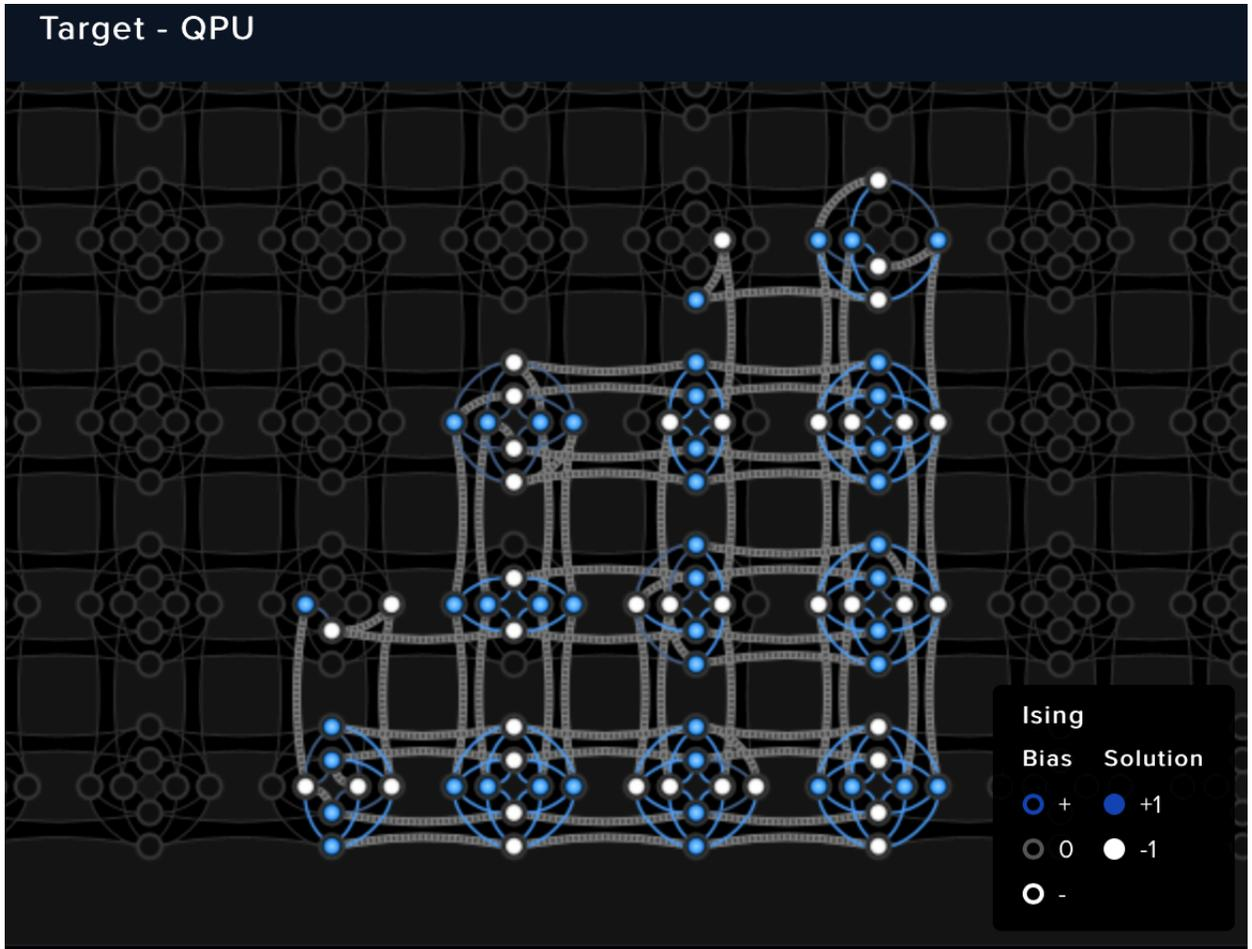
Note the gray chains connecting groups of qubits. We want each chain to contain qubits that are all the same color, that is, either all 0 or all 1. A chain is broken if it connects qubits of different colors. By enabling another option in the problem inspector (on the toolbar on the left of the screen) to show broken chains in red, we can see that all of the chains are broken:
