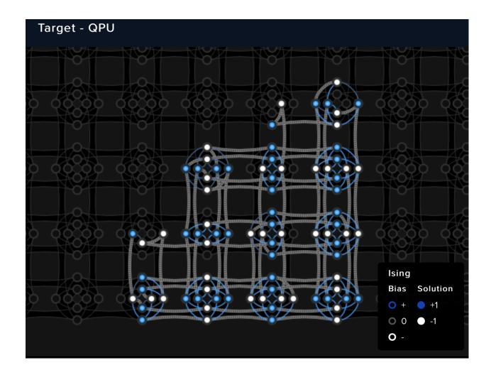
Note the gray chains connecting groups of qubits. We want each chain to contain qubits that are all the same color, that is, either all 0 or all 1. A chain is broken if it connects qubits of different colors. By enabling another option in the problem inspector (on the toolbar on the left of the screen) to show broken chains in red, we can see that all of the chains are broken:
