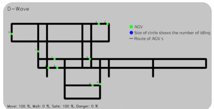
The amount of time each Automated Guided Vehicle (AGV) spent waiting for a clear route to open up was reduced by an average of 15% in this proof-of-concept.
