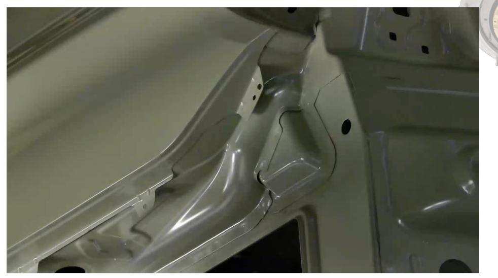
PVC Application serves to seal the gaps of joined sheets, thereby preventing the ingress of corrosive media.
